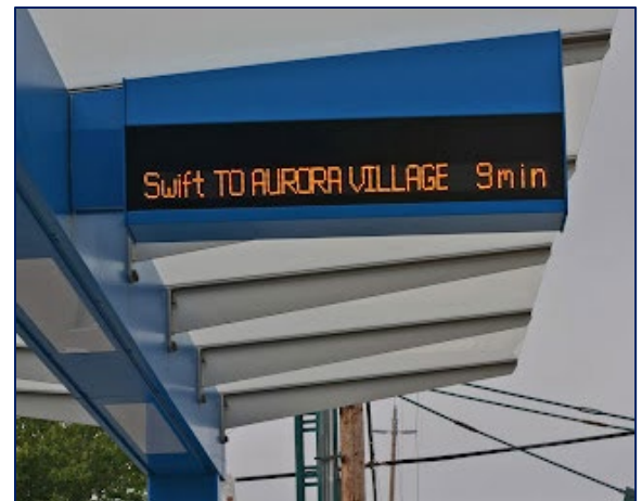
Figure 1: Real Time Arrival Board for Community Transit's Swift BRT service in Washington State (Source: Community Transit).
